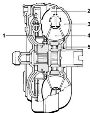
**Figure 7.3:** Hydrodynamic converter with lockup clutch
