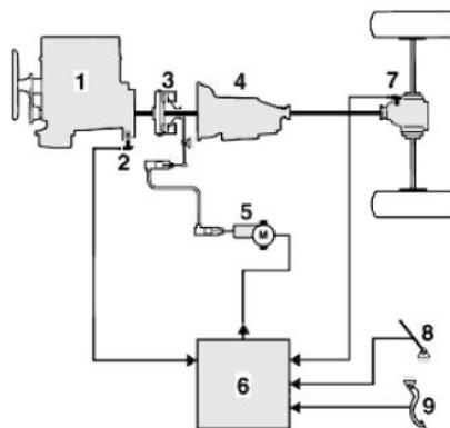
**Figure 7.2: Automatic clutch, limited to clutch actuation**
