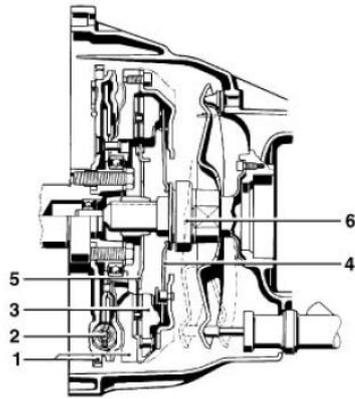
**Figure 7.1: Clutch with dual-mass flywheel**
