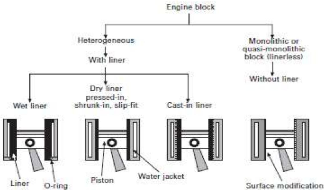
**Figure 5:** Bore design in engine blocks
