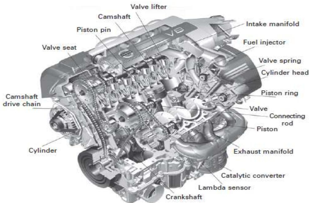
**Figure 1:** The Picture of the Cutaway of a four-stroke cycle petrol engine
