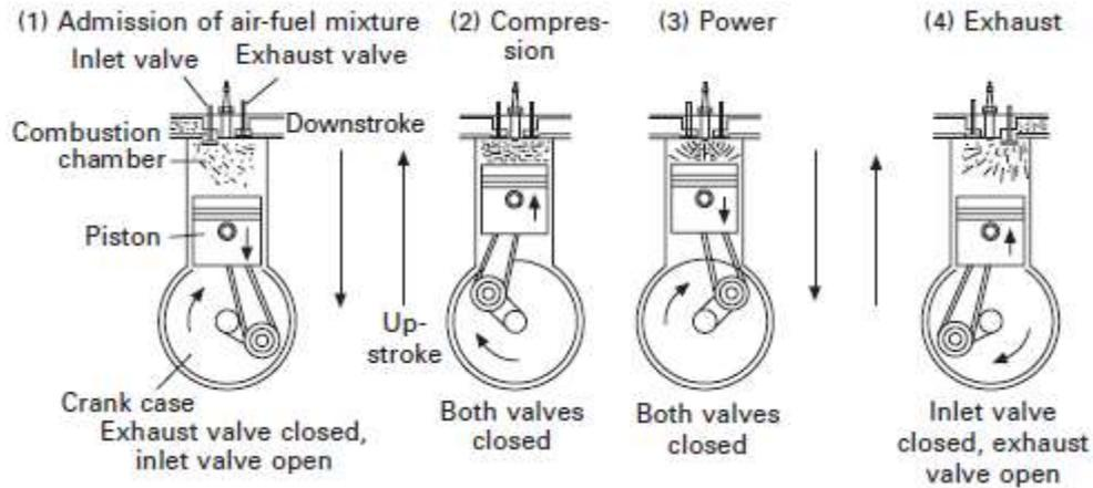
**Figure 2:** The Basic Operation of a Four-Stroke Cycle Engine
