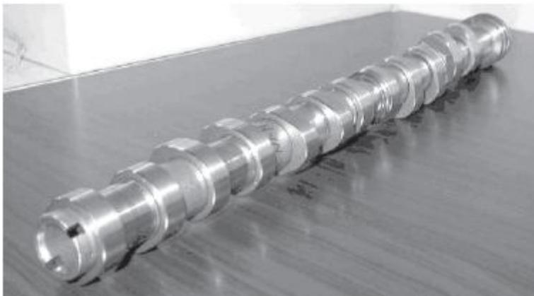
**Figure 5.13:** Assembled camshaft using mechanical joining (hydroforming)
