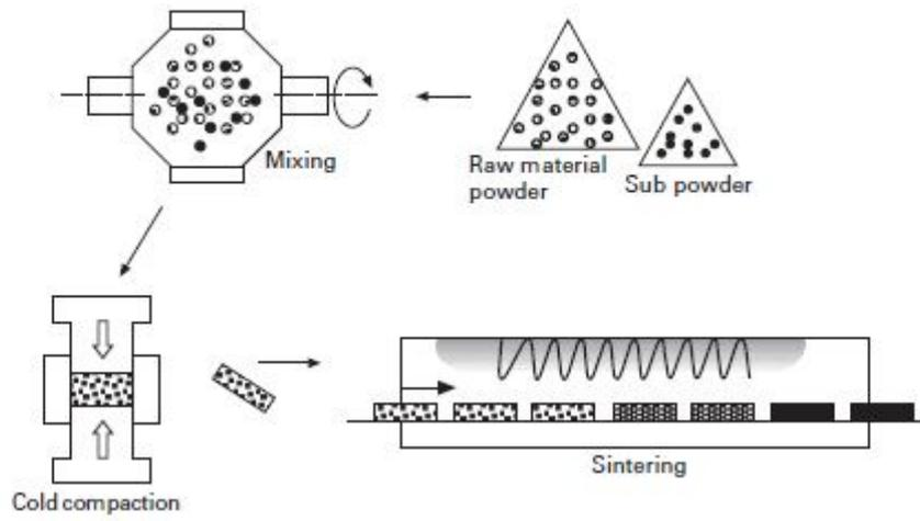
**Figure 5.15:** Powder metallurgical process.
