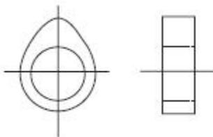
**Figure 5.14:** A cam lobe piece for assembled camshaft.
