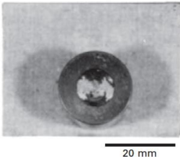
**Figure 5.7:** Flaking appearing in the valve lifter head.
