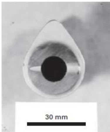
**Figure 5.9:** Camshaft cross-section at the position of an oil hole which is perpendicular to the central hole. The holes supply oil to the journal bearing.
