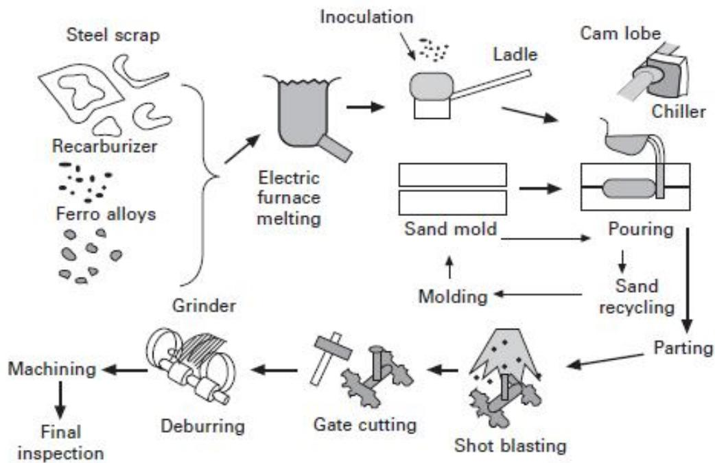
**Figure 5.10:** Casting process.
