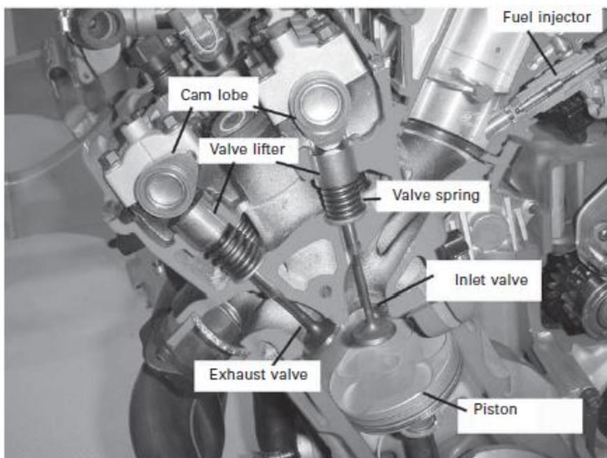
**Figure 5.1:** DOHC type valve system.
