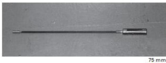
**Figure 5.11:** Gun drill. The right-hand end is a grip.
