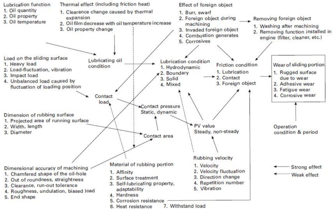
**Figure 5.6:** Tribology around the cam and valve lifter
