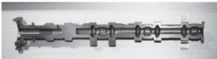
**Figure 5.12:** Chilled camshaft having a long hole as cast. To decrease the weight, the excess metal at the cam lobes is also removed.
