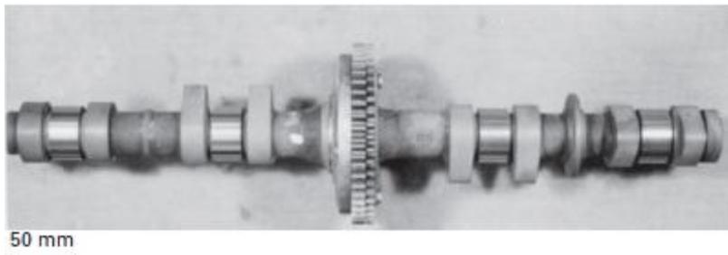
**Figure 5.4:** Camshaft installing a drive sprocket at the center
