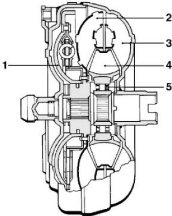
**Figure 9.3: Hydrodynamic converter with lockup clutch**
