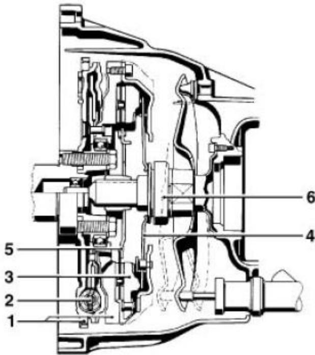
**Figure 9.1: Clutch with dual-mass flywheel**
