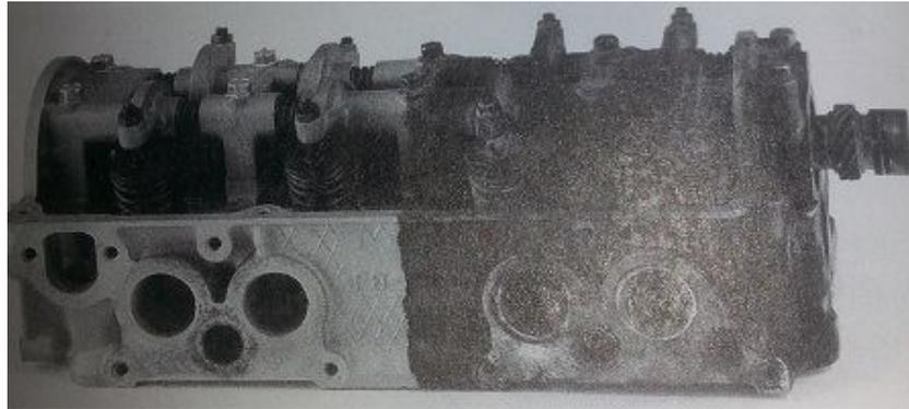
**Figure 8.5:** Half of the cylinder head was cleaned with a soda blaster
