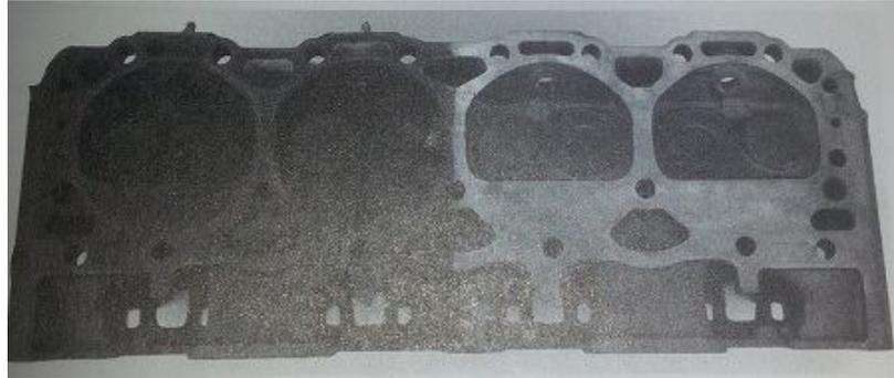
**Figure 8.3:** Part of a cylinder head cleaned with a glass bead blaster
