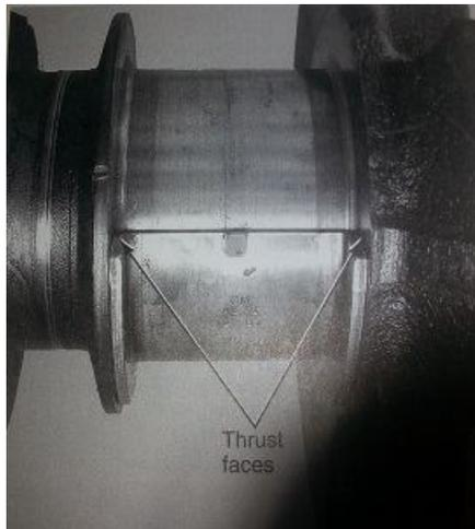
**Figure 6.0B:** Thrust insert limits the crankshaft end play
