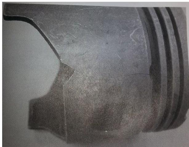
**Figure 6.1:** Cracked piston
