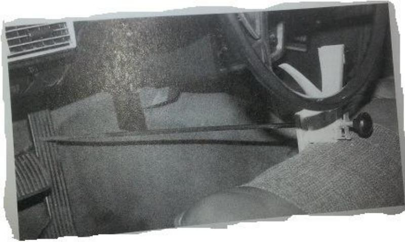
**Figure 5.11b:** A throttle depressor used to hold the throttle wide open during the compression test
