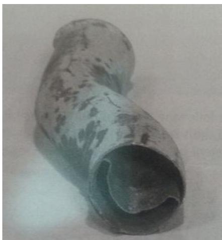
**Figure 5.10:** Collapsed exhaust pipe
