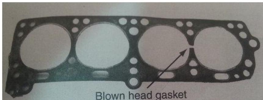
**Figure 5.7:** Blown Gasket
