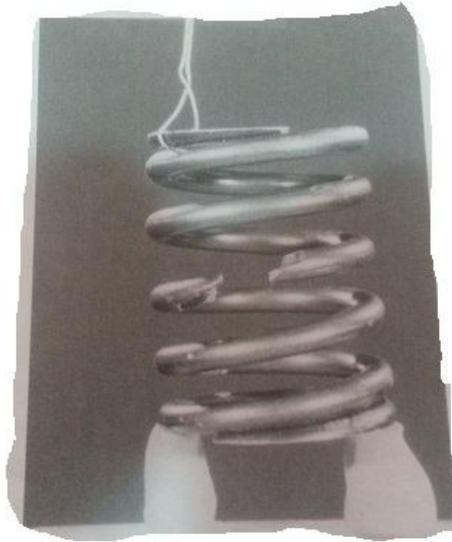
**Figure 5.8:** Broken Valve Springs
