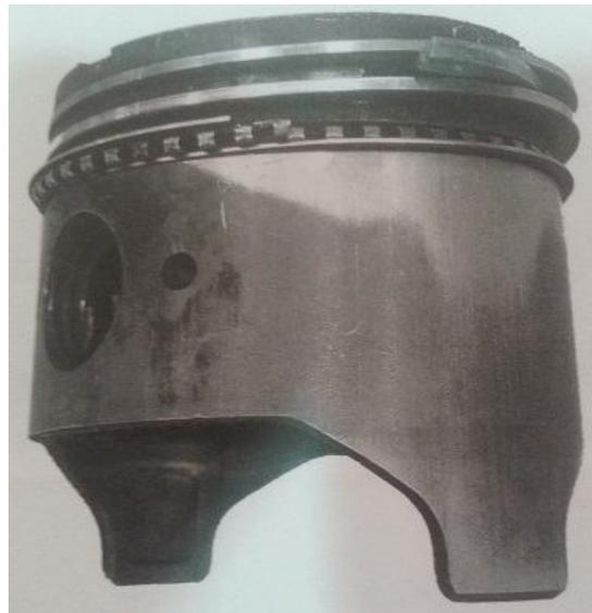
**Figure 5.5a:** Broken or worn piston rings
