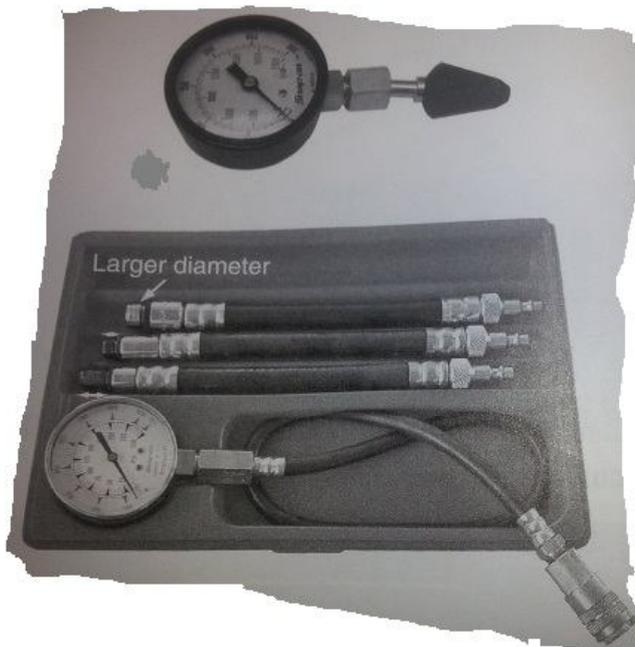
**Figure 5.11a:** Engine Compression Tester
