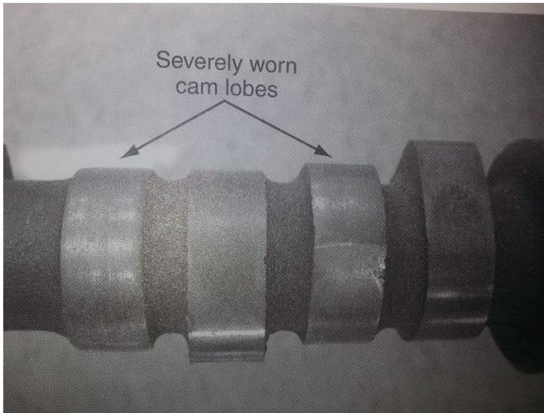
**Figure 5.9:** Worn Camshaft Lobes
