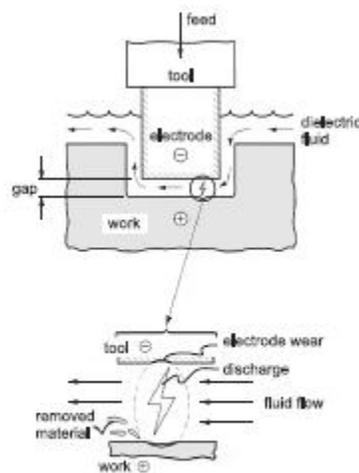
The setup of Electric Discharge Machining (EDM) process and close-up view of gap, showing discharge and metal removal.
