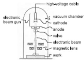
The setup of electron beam machining process.
