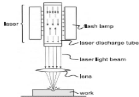
The setup of laser beam machining process.
