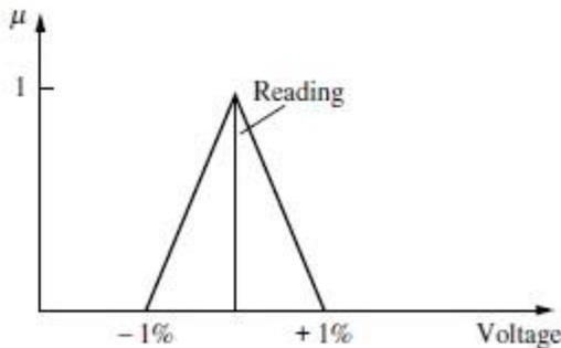
**FIGURE 5.3:** Membership function representing imprecision in “crisp voltage reading.”
