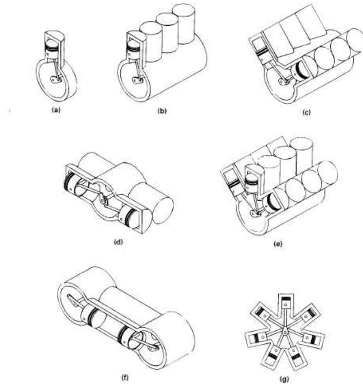
**Figure 3.1:** Engine configurations (a) Single Cylinder (b) Straight or In-line (c) V Engine (d) Opposed Cylinder (e) W Engine (f) Opposed Piston (g) Radial
