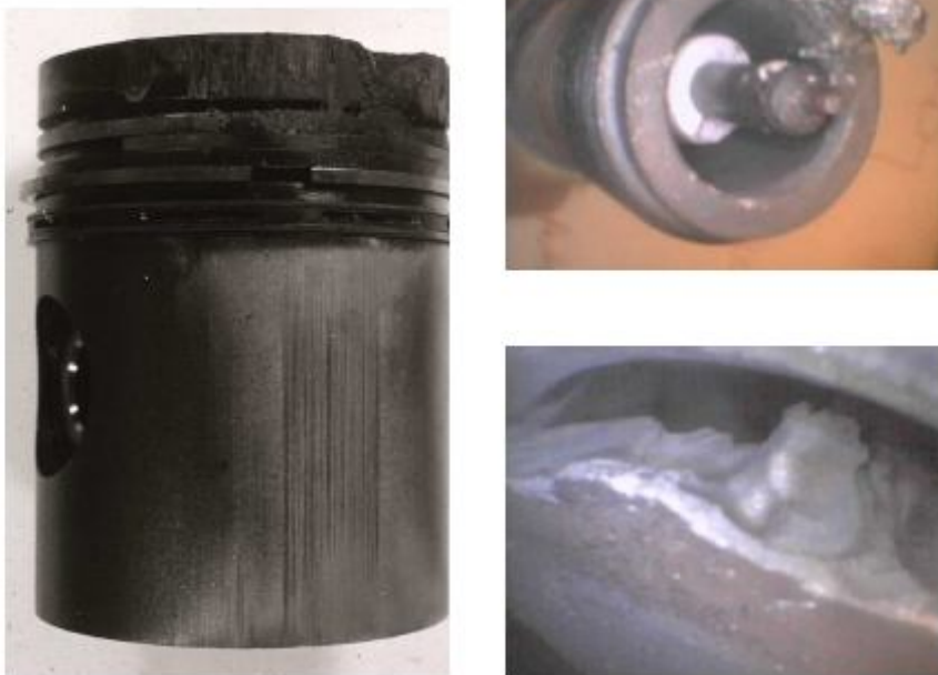
Fig. 1: Effect of abnormal combustion on engine components
