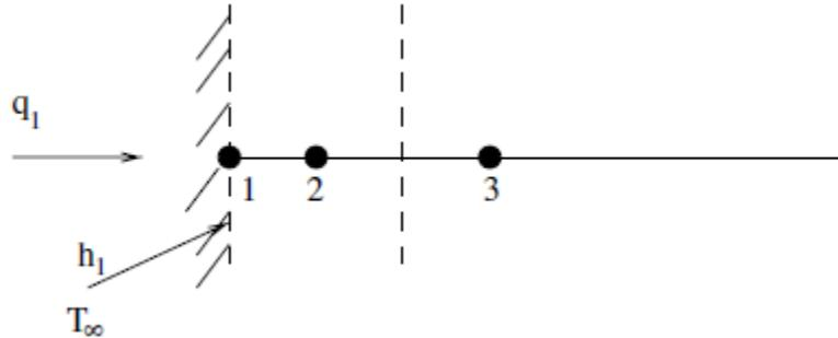
**Figure 8.** Flux boundary condition.
