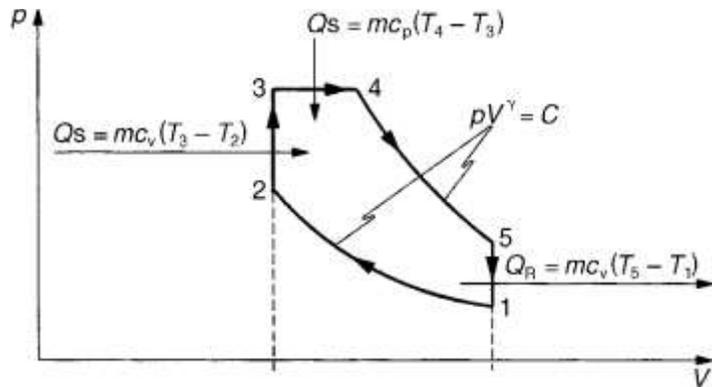
Figure 8 Mixed pressure (dual combustion) cycle
