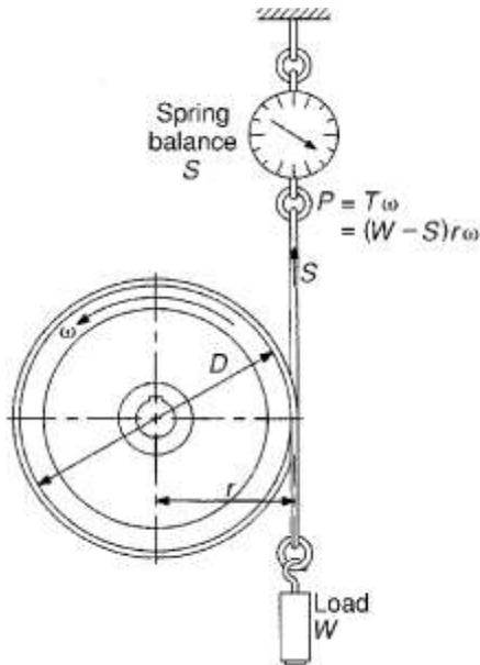
**Figure 11** Rope brake dynamometer
