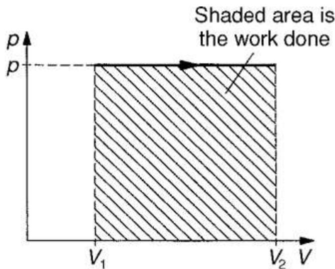
**Figure 2.3.1** *Constant pressure process*
