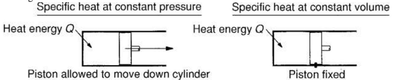
**Figure 1** Specific heats of gases.
