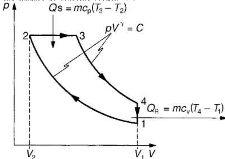
Figure 6 Constant pressure (diesel) cycle
