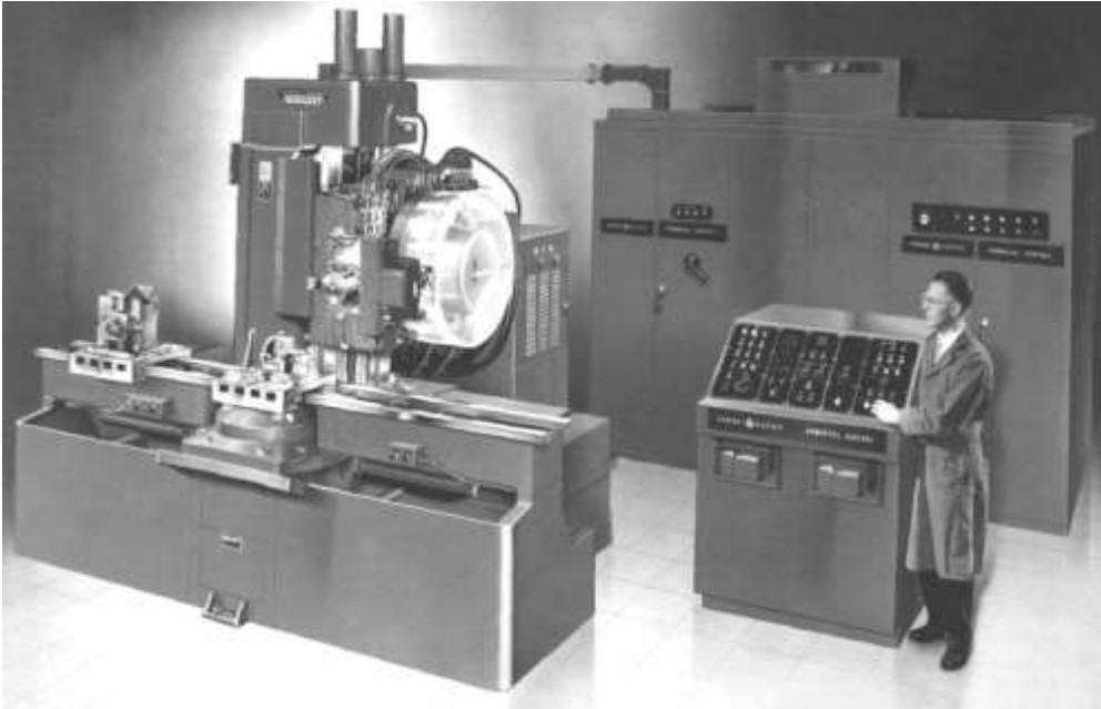
Fig-1-1959 CNC Machine: Milwaukee-Matic-II was first machine with a tool changer.
