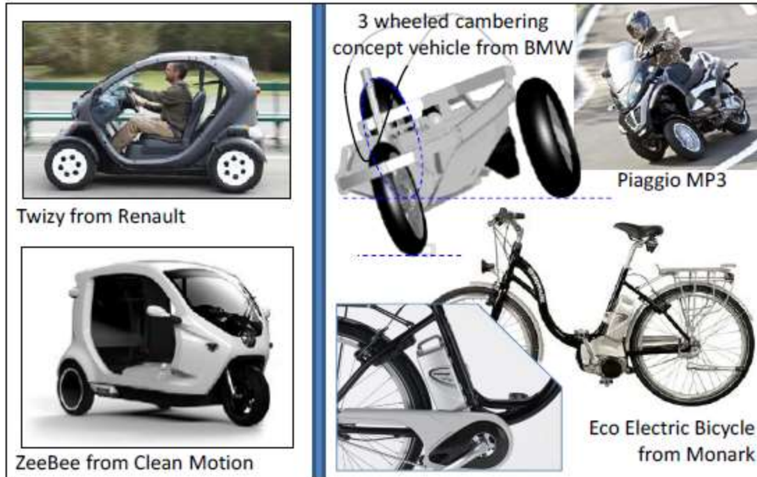
Figure 10: Examples of Urban Personal Vehicles. Left: “Roll-stiff”. Right: “Cambering“. From www.motorstown.com, www.cleanmotion.se, www.monarkexercise.se, www.nycscootering.com.
