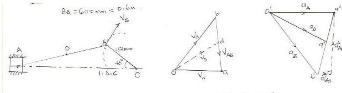
Linear velocity of B with respect to O or velocity of B.
