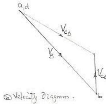
First of all, draw the space diagram to some suitable scale, as shown in fig. 2.11(a) above and the velocity diagram, as shown in fig 2.11(b) as discussed below.
