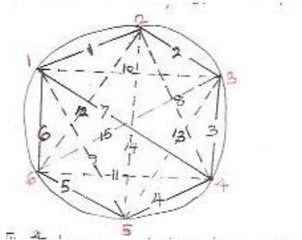
5. Joint point 2 to 4 by a dotted line to form the triangles 124 and 234. The side 2 4, common to both triangles, is responsible for completing the two triangles. Therefore the
