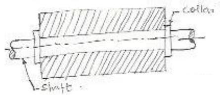
Fig.2.2. Shaft with collar in a circular hole
