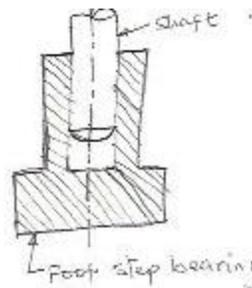
Fig. 2.4. Shaft in a foot step bearing
