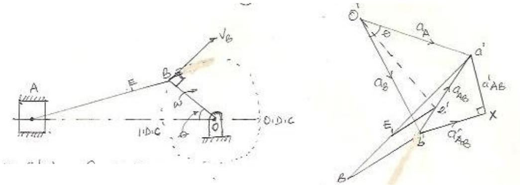
(a) Slider crank mechanism
