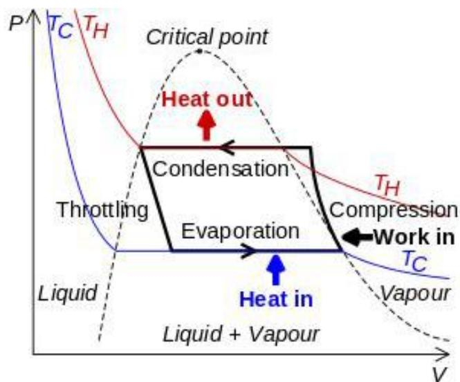
**Figure 5:** P-V diagram for a refrigeration cycle
