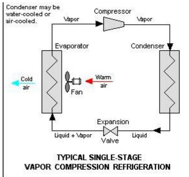
**Figure 4:** A refrigeration/Air conditioning cycle setup
