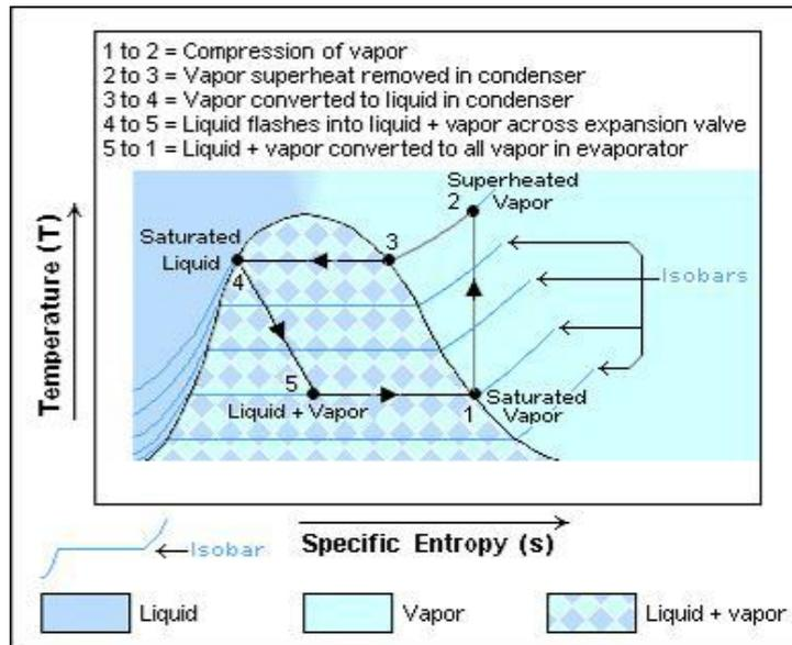
**Figure 6:** T-S diagram for a refrigeration cycle
