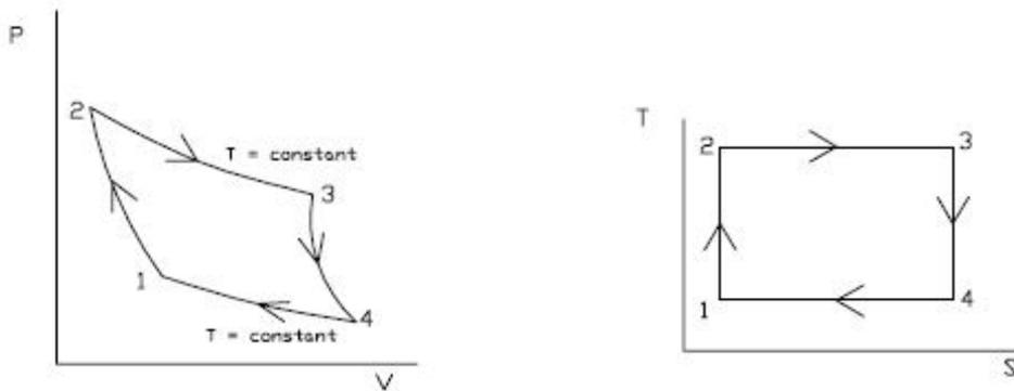
**Fig 2: The cycles of a Carnot Engine on a P-V and T-S Diagram respectively**
