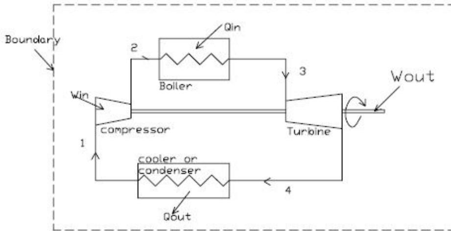
**Fig 3: Schematic diagram of a steam plant operating on a Carnot cycle**
