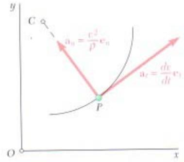
Since the velocity  $v$  of the particle is tangent to the path it can be expressed as the product of the scalar  $v$  and the unit vector  $e_t$ .
