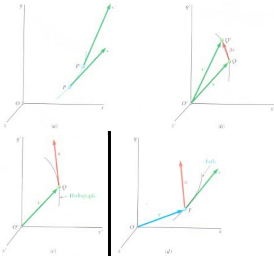
The average acceleration of a particle over the time interval  $\Delta t$  is defined as the quotient of  $\Delta v$  and  $\Delta t$ .
