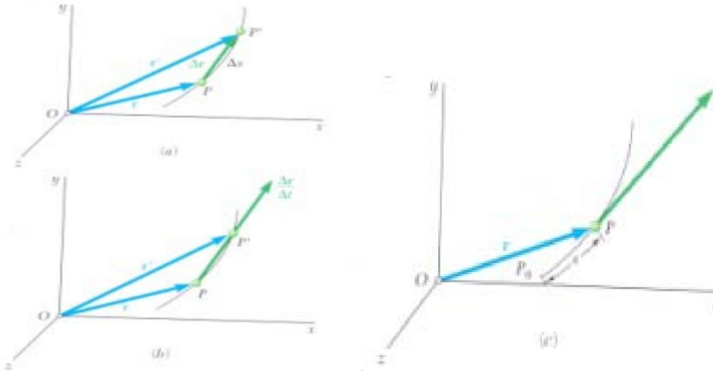
Vector  $r$  is characterized by its magnitude,  $r$ , and its direction with respect to the reference axes; it completely defines the position of the particle with respect to those axes. Hence the vector  $r$  is referred to as the position vector of the particle at time  $t$ .
