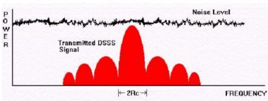
Figure 4: Direct-sequence systems combat noise problems by spreading jammers across a wideband as shown in this figure.
