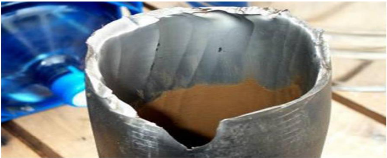
Stress Cracking Corrosion
