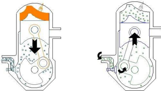
The piston starts at a lower position such that the intake port and exhaust port are opened, fuel mixture is forced in and at the same time exhaust gases are driven
