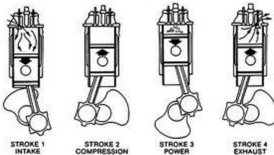
Fig. 3.1 Sequence of events in a 4 stroke cycle petrol engine
